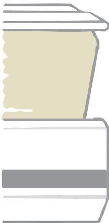
LE HAUT DE LA BOBINE CONTIENT PLUS DE LIGNE QUE LE BAS AVEC UNE RAINURE. LA BOBINE EST TROP BASSE SUR L'ARBRE PRINCIPAL. POUR Y REMÉDIER, AJOUTEZ UNE RONDELLE.
